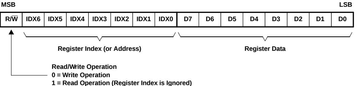
Figure 24. Control Data Word Format for MDI
