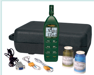
RH355 Superheat Psychrometer Kit includes meter, 33% and 75% calibration bottles, 2 temperature probes, RS232 PC cable, 4 AAA batteries and carrying case.
