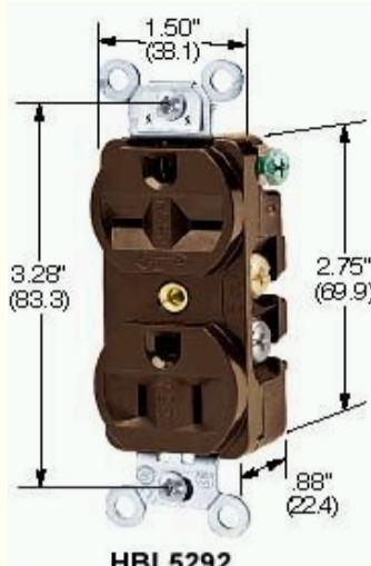
2-Pole 3Wire Grounding, 20A 125V<sup>250V</sup>R, Nylon Face, Back and Side Wired, Brown (20A Only)
