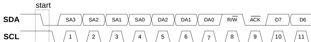
Figure 4-6. Addressing an I 2 C Peripheral
