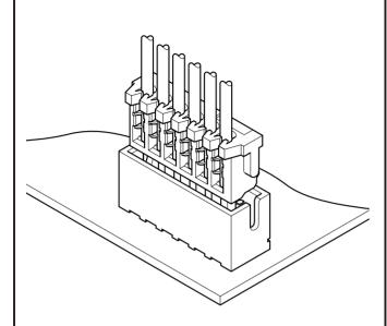
The twin U-slots (IDC slots), the 3-point insulation grip, and the distortion resistant disconnectable construction ensure a reliable connection even during severe environmental conditions.
