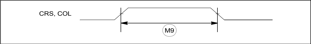
Figure 40. MII async inputs timing diagram
