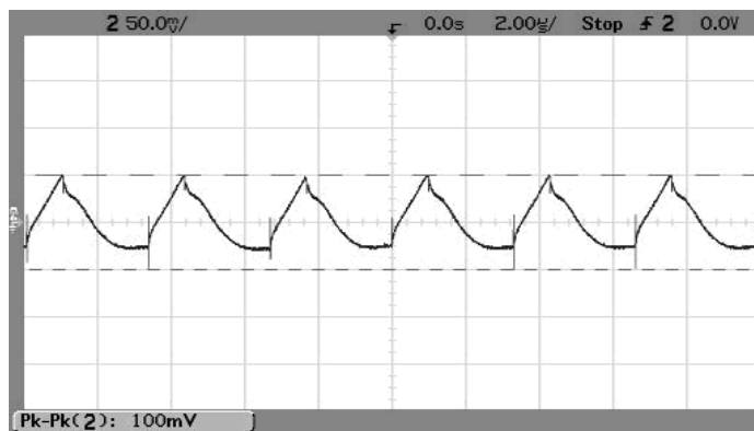
Output Ripple and Noise (V IN =12V, V OUT =3.3V, I OUT =16A, C LOAD =0, ScopeBW=100MHz)
