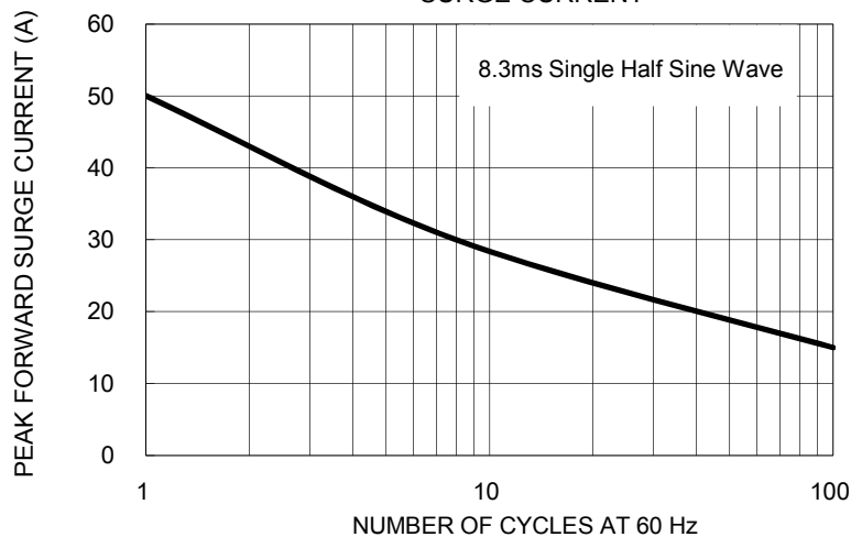
FIG. 3- MAXIMUM NON-REPETITIVE PEAK FORWARD SURGE CURRENT
