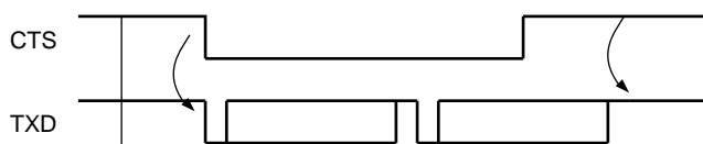
Figure 39-28. Transmitter Behavior when Operating with Hardware Handshaking
