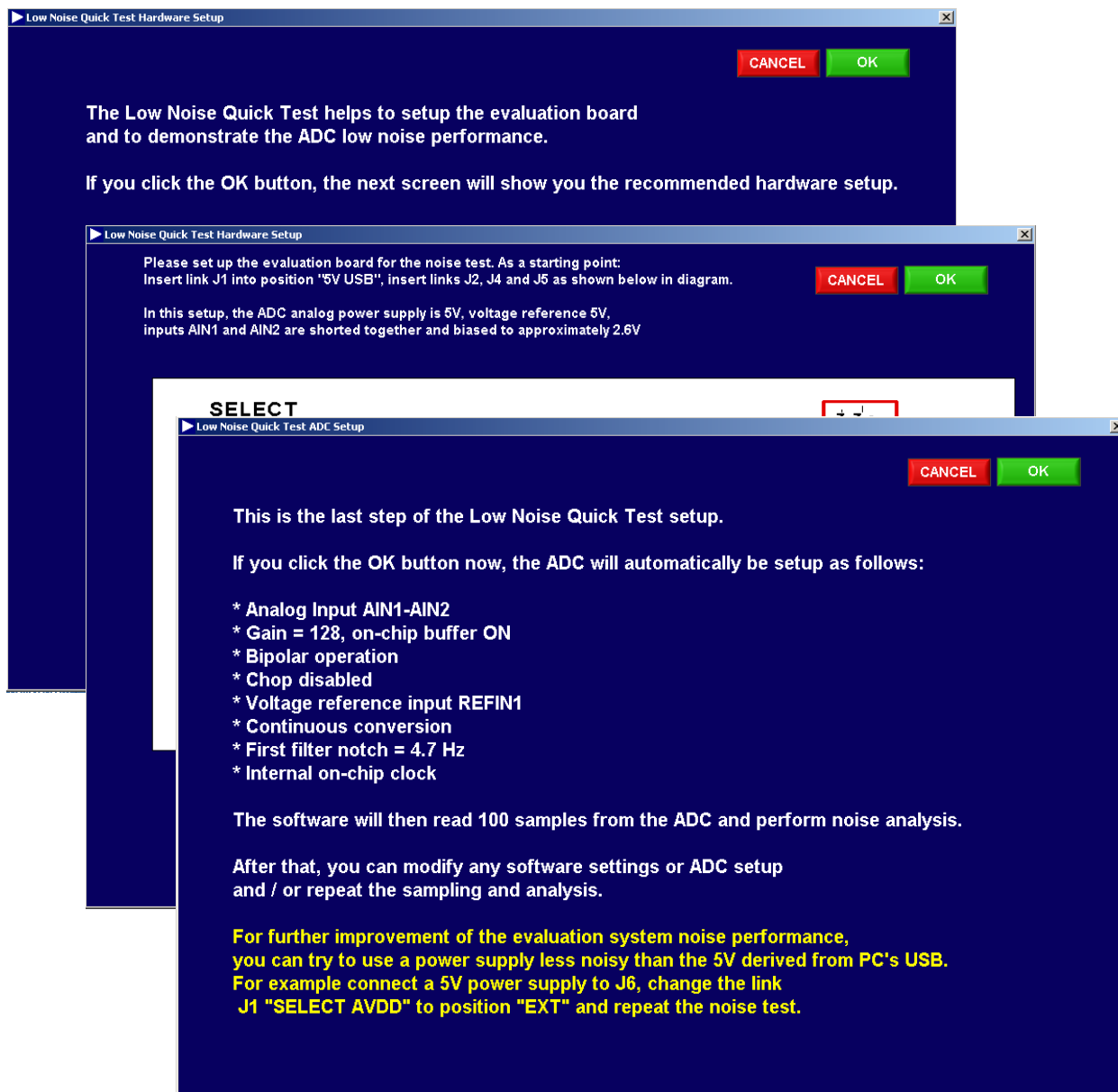
Figure 10. Low Noise Quick Test Hardware Setup
