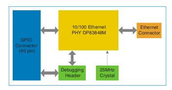
Figure below shows the connection of Ethernet MAC 10/100 Add On board with the CoreCommander board.
