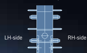
Side definition with terminals and location pins
