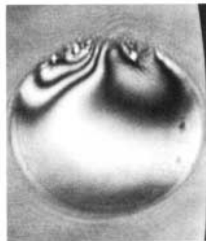
This view represents a fiber endface as viewed by an interferometer (50/125 micron coming fiber). The light/dark bands (fringes) indicate end face angle.
