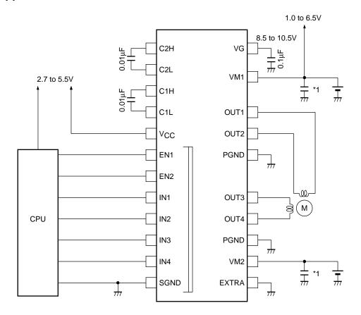
\*1 : Connect a kickback absorption capacitor directly near IC. Coil kickback may cause rise of the voltage of VM line, and the voltage exceeding the maximum rating may be applied momentarily, resulting in deterioration or damage of IC.
