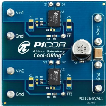
Figure 21: PI2126 Mounted on PI2126-EVAL1
