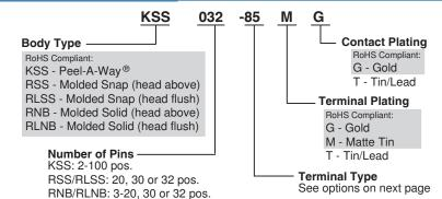
Note: Terminals plated with Matte Tin are available only with Gold plated contacts. Quick-Turn delivery is not available on products with Matte Tin plating.
