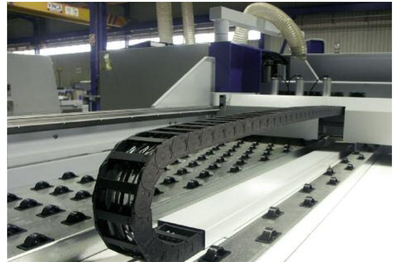
chainflex® CF130.UL for woodworking. e-chain®: E4/light
