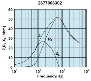
Impedance, reactance, and resistance vs. frequency.
