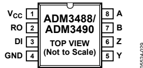
Figure 5. ADM3488/ADM3490 Pin Configuration
