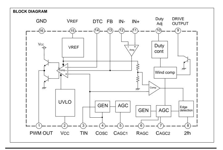
PWM IC for the synchronized deflection system control
