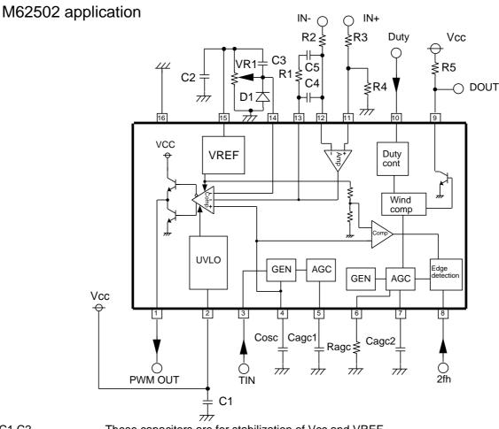
C1,C2 ----- These capacitors are for stabilization of Vcc and VREF.
