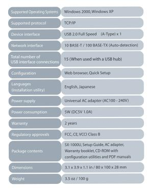
\* The SX-1000U does not currently support USB devices using isochronous data transfer mode, such as web cameras & speakers.
