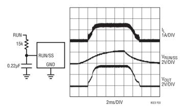
Figure 3. To Soft-Start the LTM8023, Add a Resistor and Capacitor to the RUN/SS Pin
