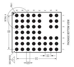
NOTES: 1. DIMENSIONING AND TOLERANCING PER ASME Y14.5M-1994 2. ALL DIMENSIONS ARE IN MILLIMETERS
