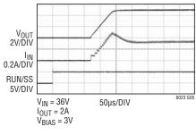
36V<sub>IN</sub> Start-Up Waveforms  $(3.3V_{OUT})$
