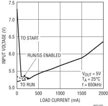
Figure 2. The LTM8023 Needs More Voltage to Start Than to Run
