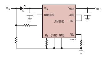
Figure 4. The Input Diode Prevents a Shorted Input from Discharging a Backup Battery Tied to the Output. It Also Protects the Circuit from a Reversed Input. The LTM8023 Runs Only When the Input is Present.
