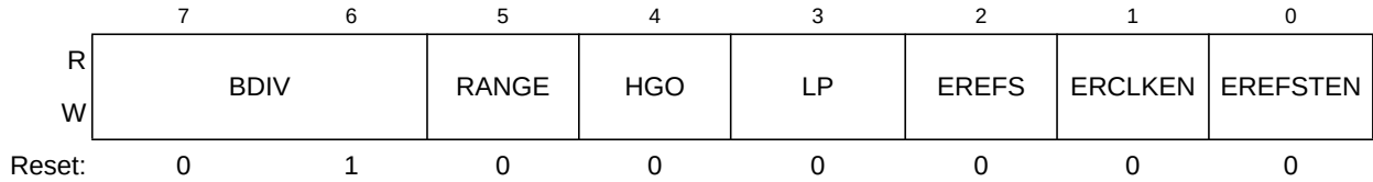
Figure 11-4. ICS Control Register 2 (ICSC2)
