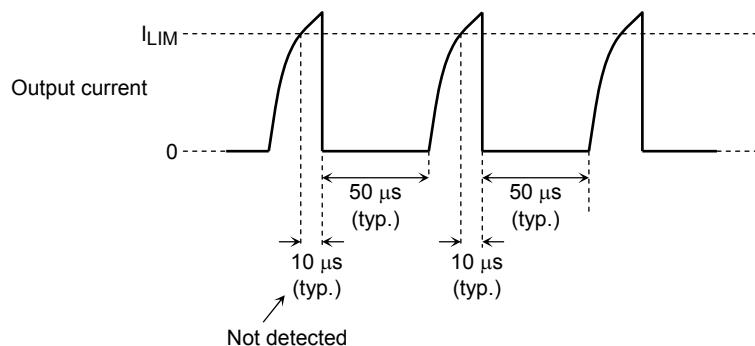
The over-current threshold is a target spec. It varies in a range from approximately 1.5 A to 3.5 A.
