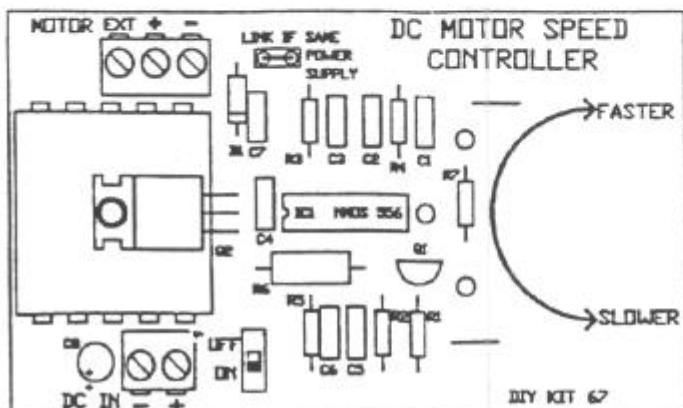
timer/oscillator, NE556. This IC has two 555 timers in one 14-pin IC package.
