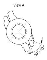
Hole arrangement View in mounting direction
