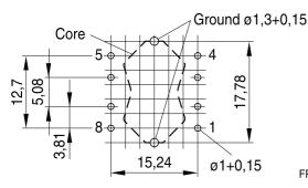
Hole arrangement View in mounting direction
