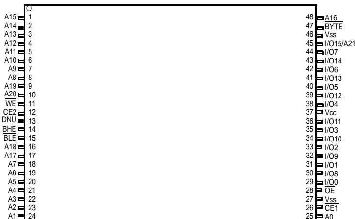
Figure 1. 48-pin TSOP I pinout (Front View) [1, 2]
