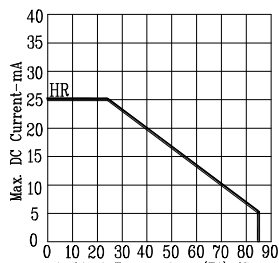
Fig5. MAX. ALLOWABLE DC CURRENT VS. AMBIENT TEMPERATURE.
