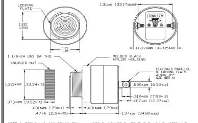
NOTE A: TERMINALS-032 BRASS TIN PLATED, TAPPED FOR #6-32 SCREW. TWO #6-32 NICKEL PLATED BRASS SCREWS INCLUBED. WILL ACCEPT 1/4\* QUICK CONNECT. NOTE B: MOUNTING- REMOVE BLACK PLASTIC NUT AND INSERT THREADED FRONT THROUGH 125' HOLE PUNCHED IN PANEL, IF DRIENTATION IS NEEDED, NOTE LOCKING FLATS ON DRAVING, SCREW NUT BACK ON. DO NOT OVERTIGHTEN.
