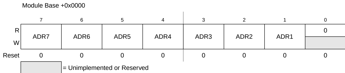
Figure 10-3. IIC Bus Address Register (IBAD)
