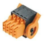
Female connector with integral cross-connection and clear printing for uninterrupted relaying of potential at full current-carrying capacity with the maximum cable cross-section. The cross-connection is positioned vertically between the poles of rows directly on top of each other. Conductor connection with tension clamp system with straight outlet and 3.5 mm pitch. Flange and release lever available. Packed in cardboard box.
