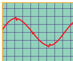
Active Tracking® Filtering virtually eliminates high-voltage transients.
