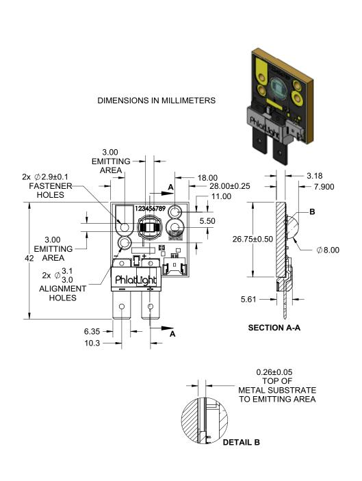
Recommended connector for Anode and Cathode: Panduit Disco Lok™ Series P/N: DNG14-250FL-C For detailed drawing please refer to DWG-001277 document
