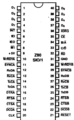
Figure 4. 40-pin Dual-In-Line Package (DIP), Pin Assignments
