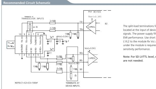
The split-load terminations for ECL signals need to be located at the input of devices receiving those ECL signals. The power supply filtering is required for good EMI performance. Use short tracks from the inductor L1/L2 to the module Rx Vcc and Tx Vcc. A GND plane under the module is required for good EMI and
