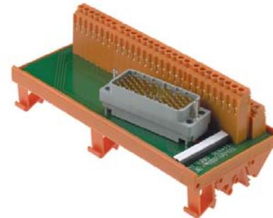
Weidmuller's passive interface units are used for adapting hermaphrodite ELCO multi-pole connectors, for input and output, to screw terminal systems. The hermaphrodite contact is a fork-type contact that is identical in design on both sides of the connection, but with one fork turned through 90° to engage with the other.
