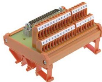
Users have a choice between screw, tension clamp or spade connections for connecting actuators and/or sensors. As an option, interface units can also integrate additional functions such as status indicator, signal disconnector, fuses or shielding. Identification systems make it easier to trace the signals to the corresponding element.
