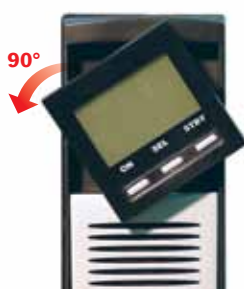
2. Rotate the mimic panel and insert it into position
