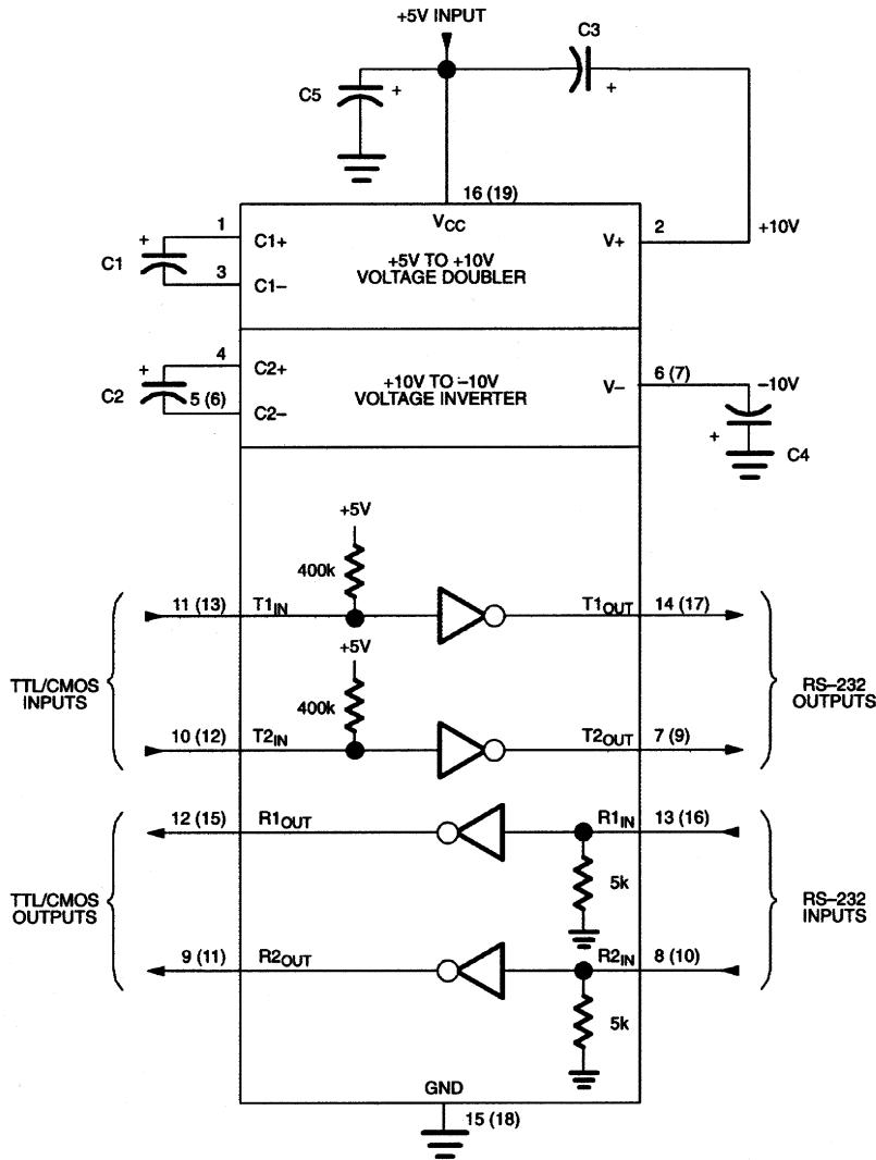
NOTE: C5 is a recommended decoupling capacitor which is the same value as C1, C2, C3, and C4.
