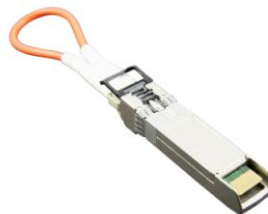
Figure 8-1 Optical SFP+ Loopback Fixture
