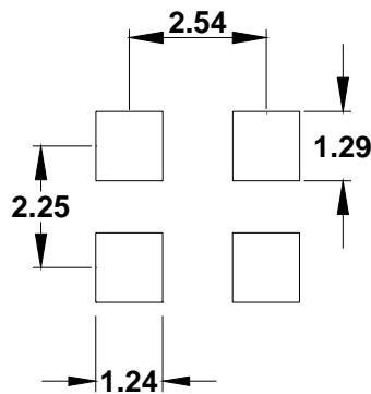
Note: XPRESSO HCMOS XOs are designed to fit on industry standard, 4 pad, layouts.
