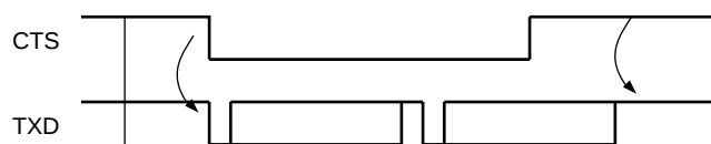
Figure 34-29. Transmitter Behavior when Operating with Hardware Handshaking
