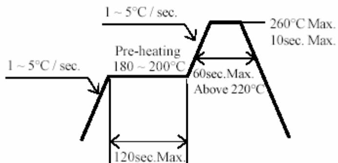
2. Reflow soldering should not be done more than two times.
