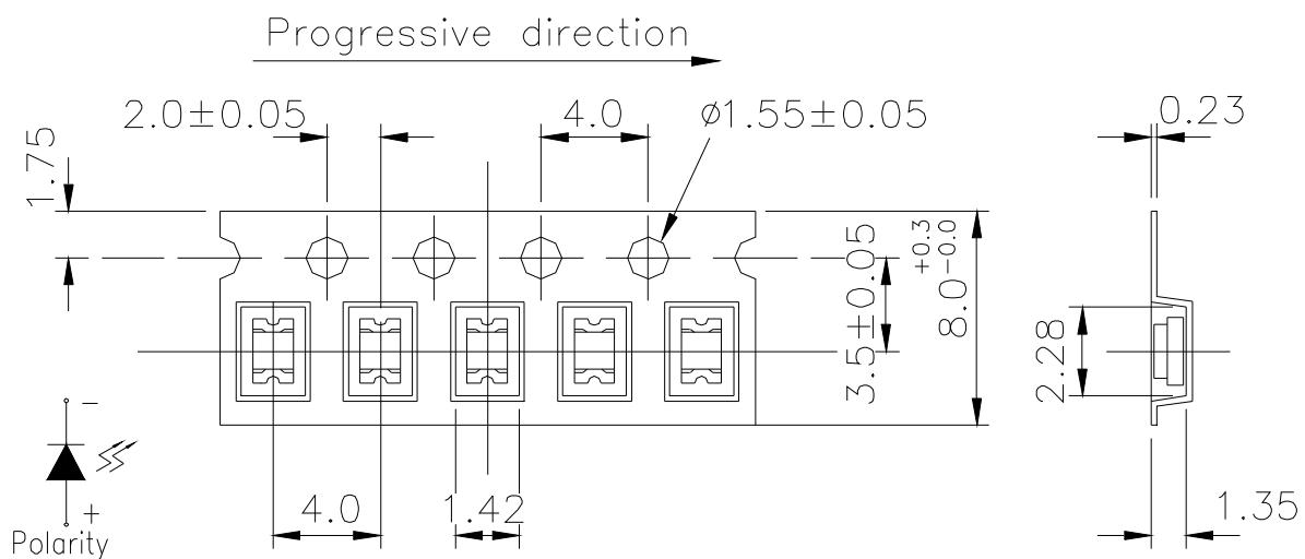
**Note:** The tolerances unless mentioned is ±0.1mm , Unit = mm
