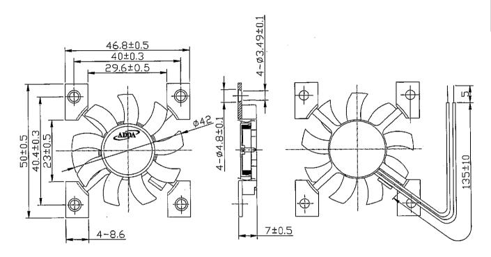
LEAD WIRES: UL 1571, AWG28, L = 135 +/- 10 MM Red = positive; Black = negative.
