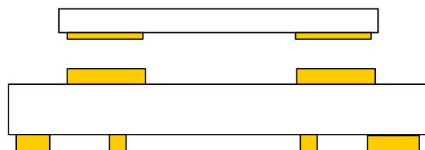
Figure 20. Correct PCB Top Metal Pattern Under Package
