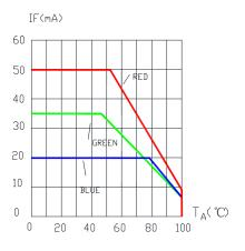
MAXIMUM FORWARD DC CURRENT VS, AMBIENT TEMPERATURE.
