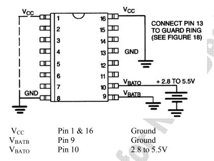
The  $V_{BATO}$  pin is normally connected to any standard 3 V lithium cell or other energy source. The Battery Operate mode also minimizes the power-consumption in applications where battery backup is not required and the  $V_{BATO}$  lead is directly connected to the system's 5V supply.
