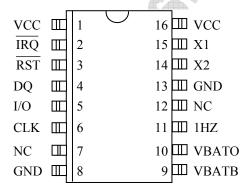
16-PIN DIP (300 MIL) 16-PIN SO (300 MIL) 16-PIN SSOP (208 MIL)
