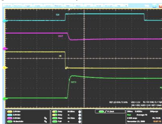
Figure 20: Turn ON output current characteristics (1)
