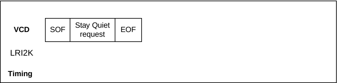
Figure 41. Stay Quiet frame exchange between VCD and LRI2K
