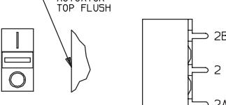
Markings are reversed on V702 and V802 models. Actuator color is red with white markings (std.).
