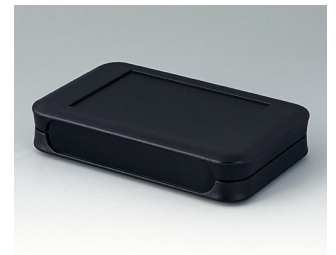
A9052209 SOFT-CASE L PMMA (IR) (UL 94 HB) black RAL 9005 2.87"x4.61"x0.94" IP 54 opt., IP 40
